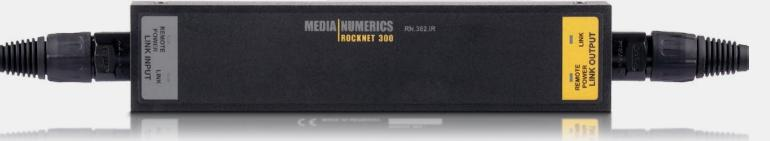
The RN.362.IR Inline Repeater extends the length of the CAT5 based infrastructure between two RockNet 300 devices to a maximum of 450m (1,500ft). It utilizes the standard network interface incorporating Media Numerics® proprietary core technology. The Inline Repeater can be remotely powered by any 19" RockNet 300
